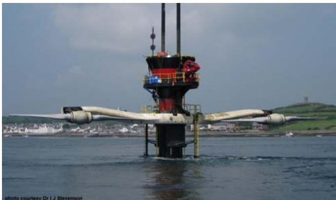
The SeaGen tidal turbines generate power from sea currents. The high density of seawater compared to wind allows for a much smaller system.
